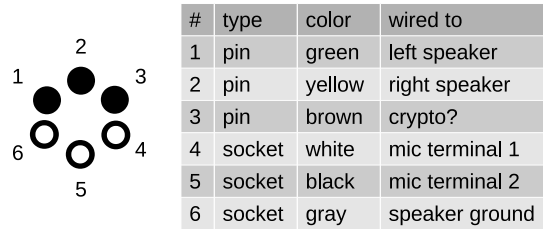
Figure 3: Lemo pin assignment
